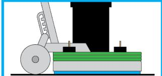
**NEW:** Guide Wheels constantly engaged to the floor for stability
